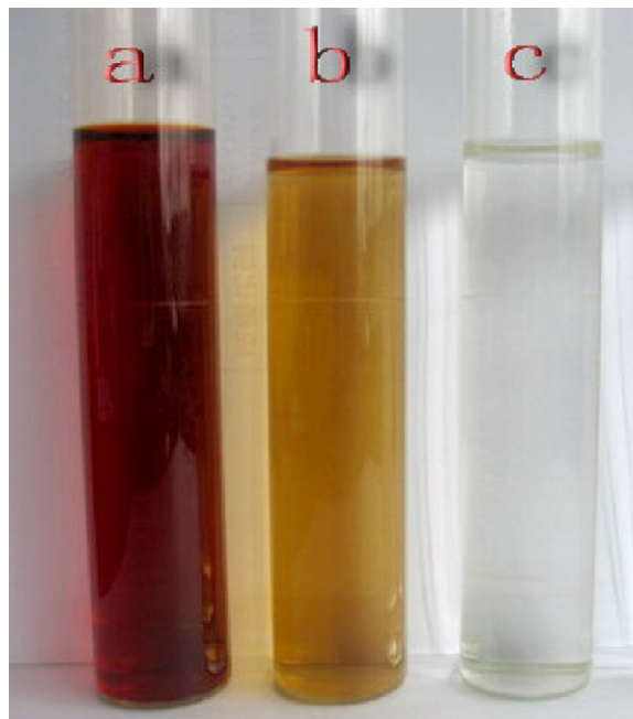
Fig. 6. Color changes of solutions: (a) original 500 \text{ mg L}^{-1} Orange II solution; (b) solution after degraded on a \text{Ti/SnO}_2\text{-Sb} electrode; and (c) solution after degraded on a \text{Ti/SnO}_2\text{-Sb-Ce} electrode.
